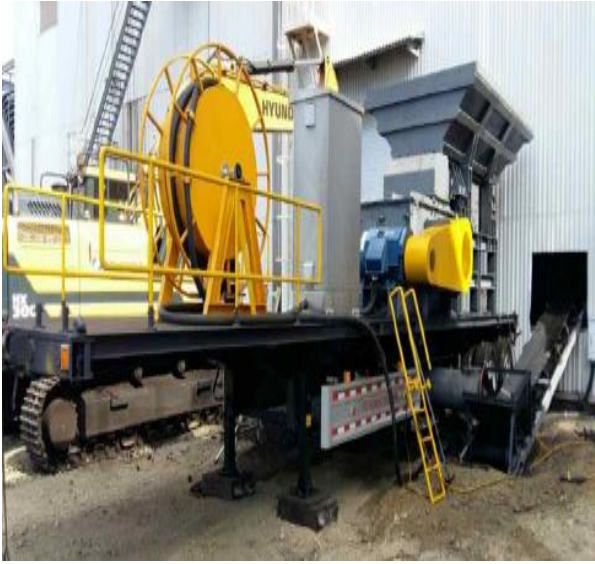
Movable Coal Crusher
